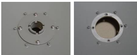
Remove Center Dish Flange
